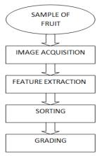
Fig. 1 Flow chart of sorting and grading process
