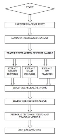
Fig. 2 Flow chart of design of proposed system for quality detection of fruit by using ANN
